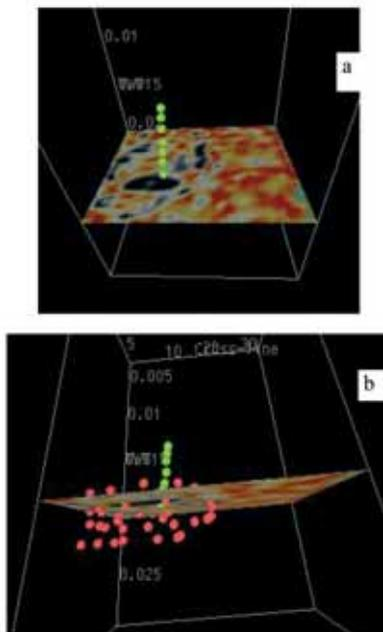
Figure 8 Time slice 20 ns, cube acquired at 13h40 a) tube position b) tube position and Interpreted water bubble
