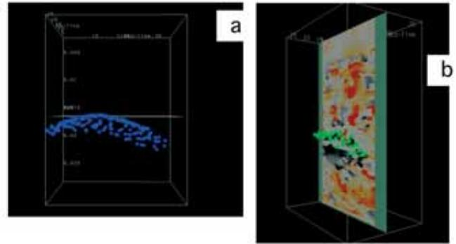
Figure 5 Picked hyperbolas thanks to (a) GPR data (b) after Dip attribute computation. With this approach to interpretation on two data sets, hyperbolas can now be picked in all profiles.
